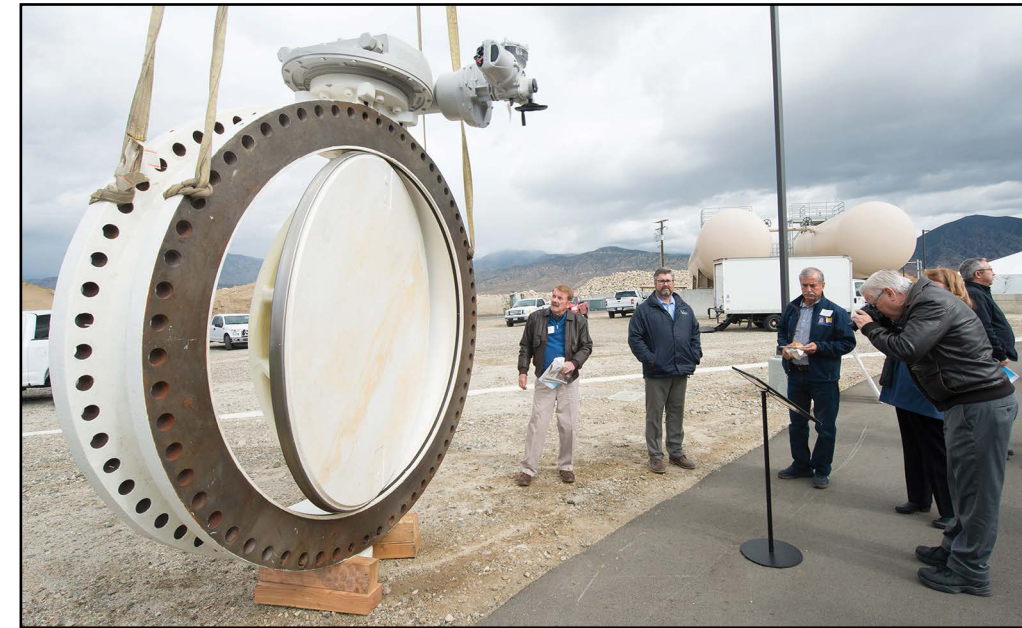
In this photo taken on February 22, 2018, a butterfly valve is on display during a celebration of the East Branch Extension project at Citrus Reservoir and Citrus Pump Station, located in Mentone, California. A valve is a device that controls the passage of water through pipelines. They are important for water infrastructure because they act as the primary line of defense when there is an issue in the pipeline, and water flow needs to be isolated to prevent impacts to adjacent infrastructure. The East Branch Extension conveys water to the east side of San Bernardino County. Source: Department of Water Resources
