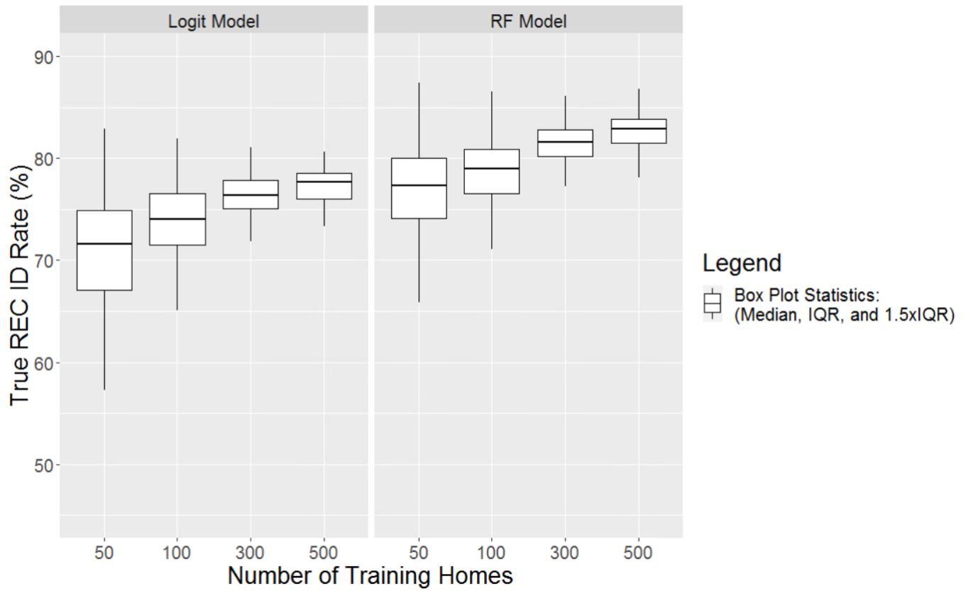
Figure 8. Distributions of classification sensitivity for different training-set sizes (50, 100, 300, and 500 in each category AC and REC) and for two classification methods, logit and random forest, trained using all non-energy-based predictors. Bar and whisker plots show median value, interquartile range (IQR), and 1.5 times the IQR.
