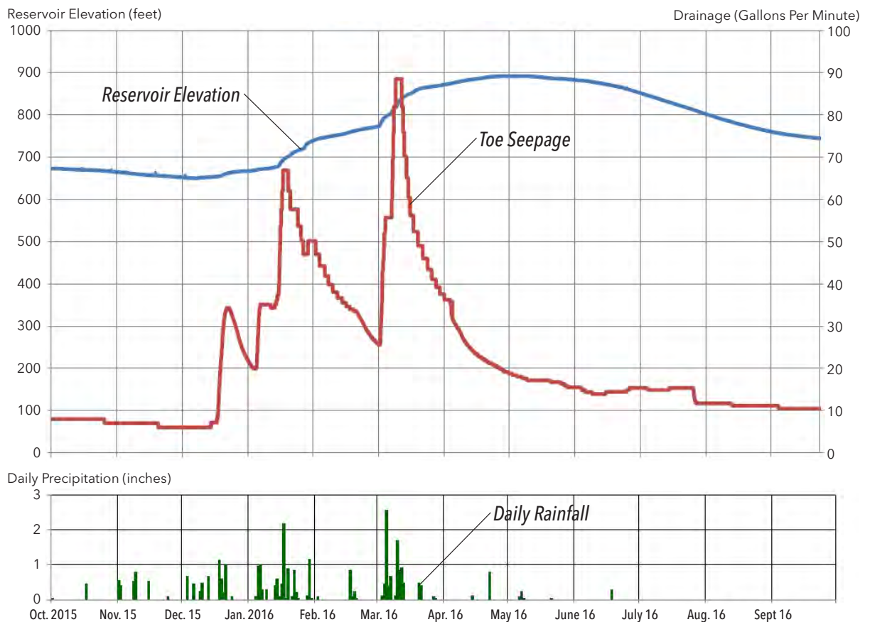
FIGURE 9. Water Year 2015-2016 Rainfall and Seepage Measurements made at the Seepage Weir Located at the Base of Oroville Dam.
