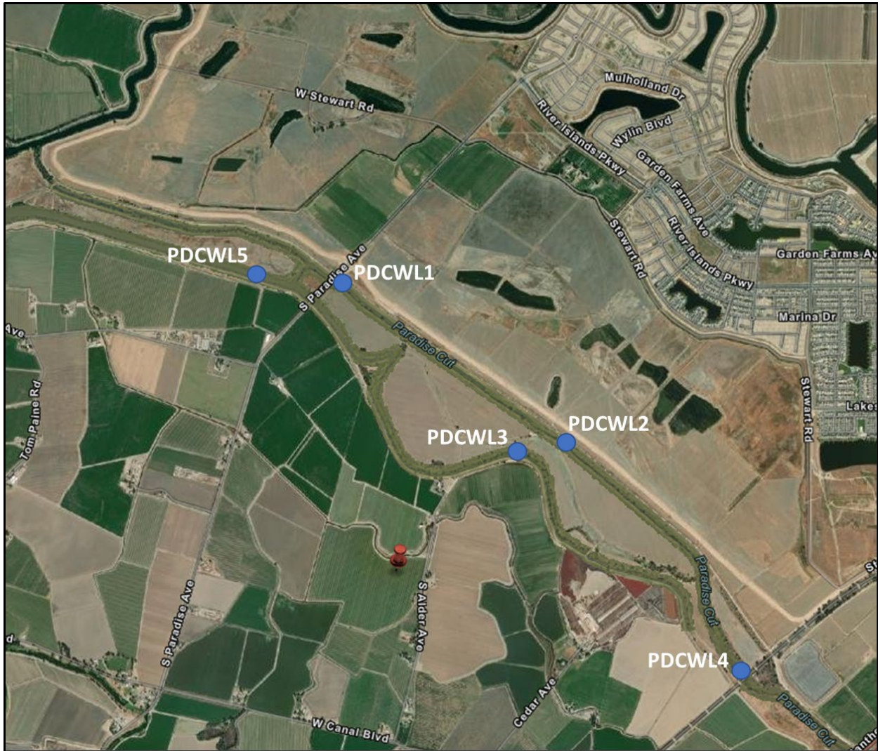
Figure 25. Map of Continuous Water Level Monitoring Sites in Paradise Cut that Provide Supporting Data for the Pescadero Tract Circulation Study; Sites Denoted by Blue Circles
