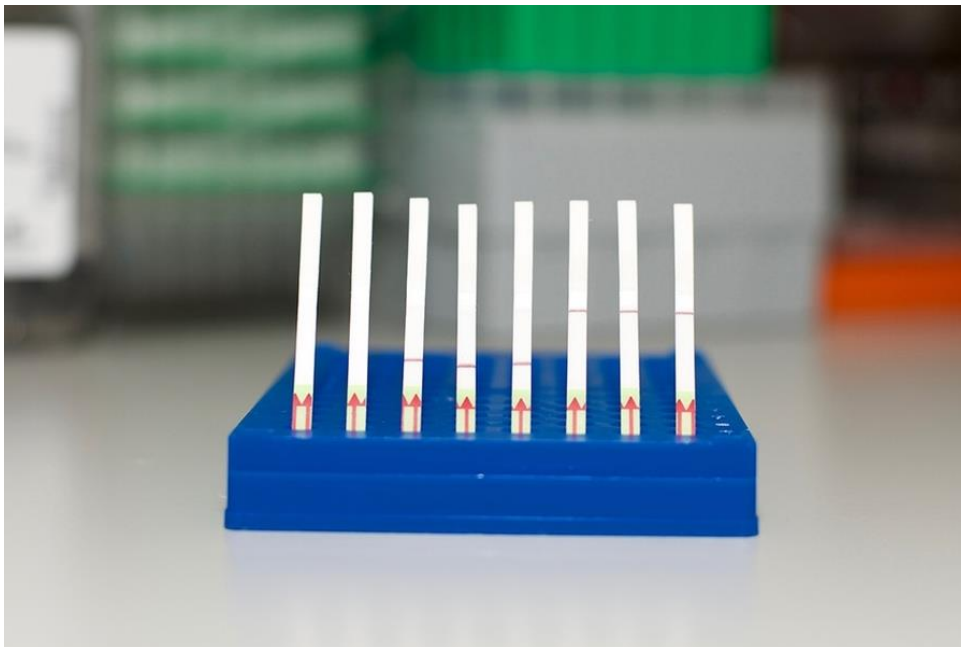
Figure 15 Photograph of SHERLOCK Technology Applied Using Test Strips; the Presence or Absence of a Line on Each Strip Visually Indicates Genetic Identification
