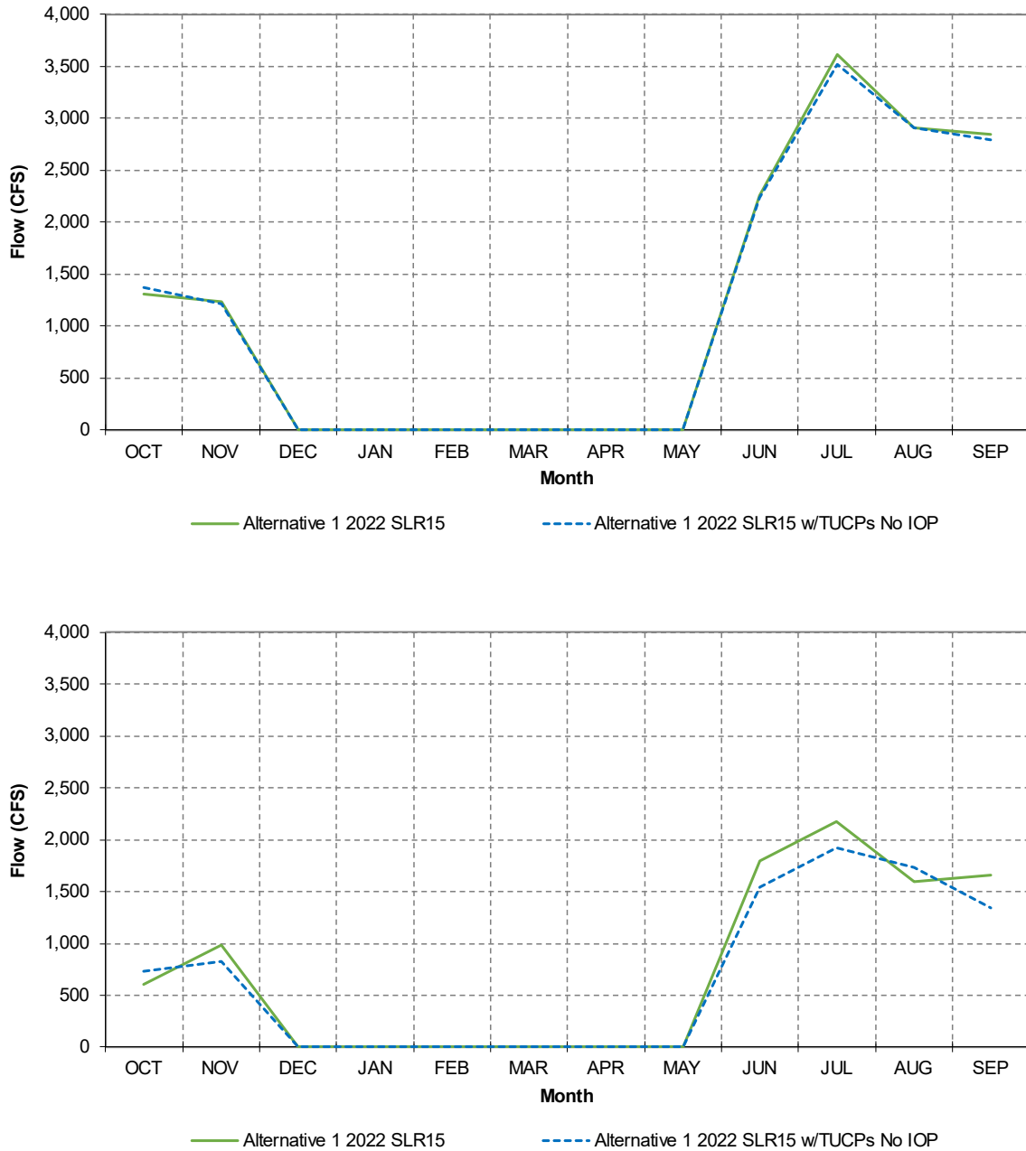
Figure 4I-I-13. Monthly Long-term (Top) and Critically Dry Water Year (Bottom) Average Delta Cross Channel Flow for Alternative 1 under Future Climate Centered around 2022 with 15 cm of Sea Level Rise (with and without TUCPs and the IOP)
