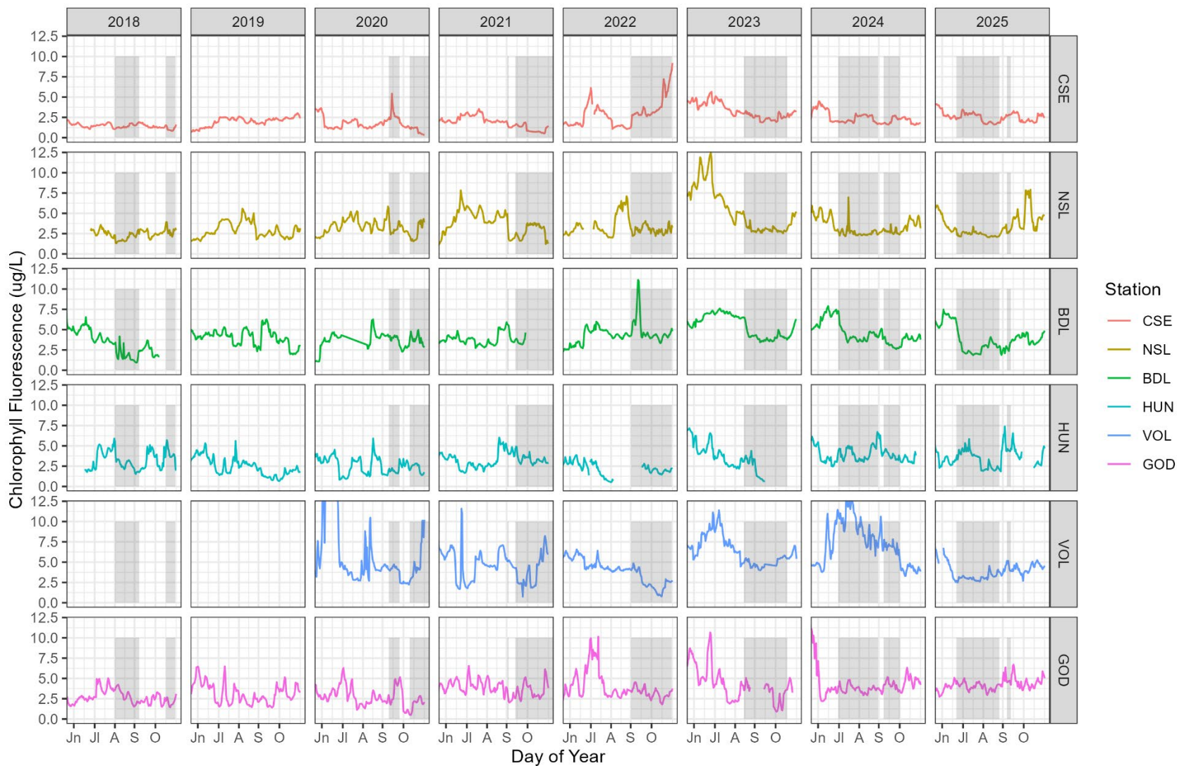
Figure 15. Time series of chlorophyll fluorescence at one station in the lower Sacramento River (CSE) and several stations in Suisun Marsh during the summer and fall of each year (June–October). Gray boxes indicate time periods when the SMSCG were operating.
