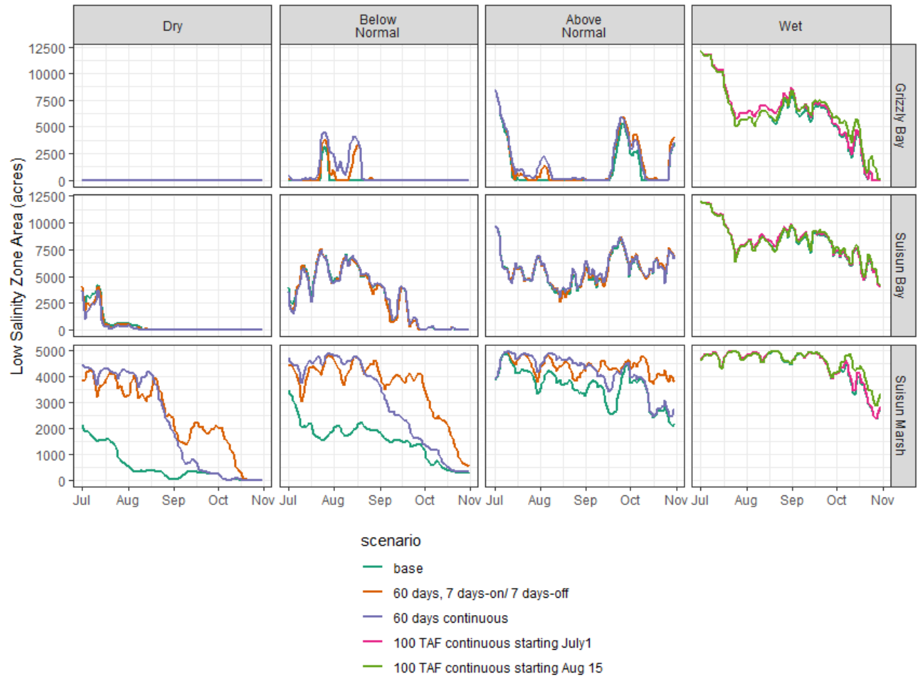
Figure 14. Low Salinity Zone area in Suisun Marsh, Suisun Bay, and Grizzly Bay for different SMSCG operational scenarios and different water year types.
