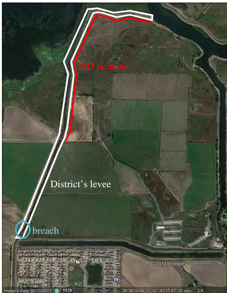
Figure RC-1. Location of Contra Costa County Flood Control and Water Conservation District Levee (in white), the Ironhouse Sanitary District pipeline in landside levee toe (in red), and the approximate location of the levee breach to route Marsh Creek onto the parcel (in blue).
