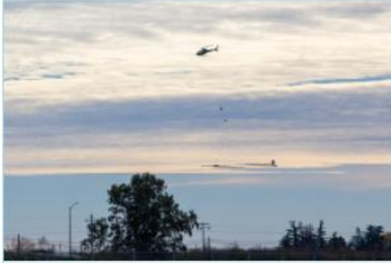
Flyover of a helicopter performing an Airborne Electromagnetic Survey.
