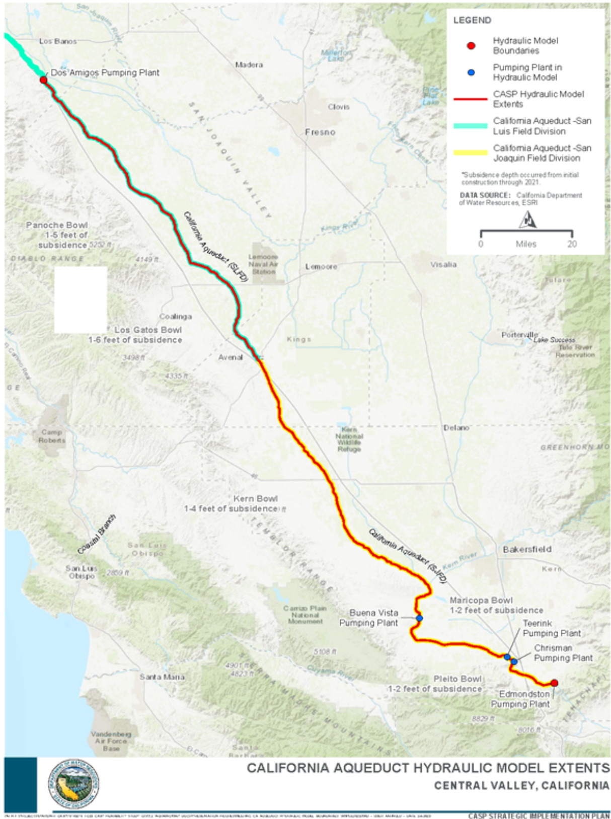
Figure 3-1. California Aqueduct Hydraulic Model extents
