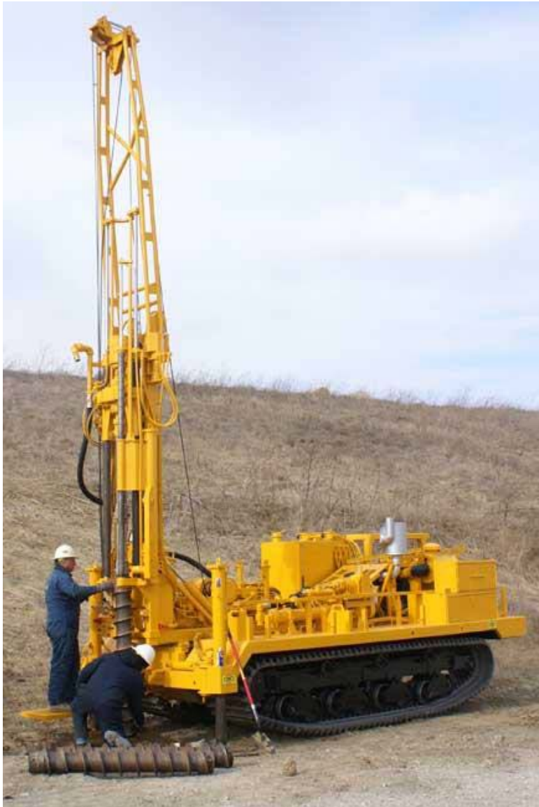
Figure 3. Truck-mounted Rotary Drill Rig
