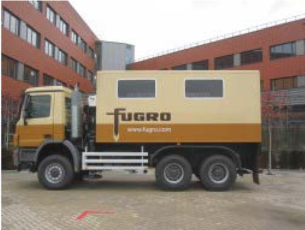
Figure 5. Cone Penetrometer Testing Rig
