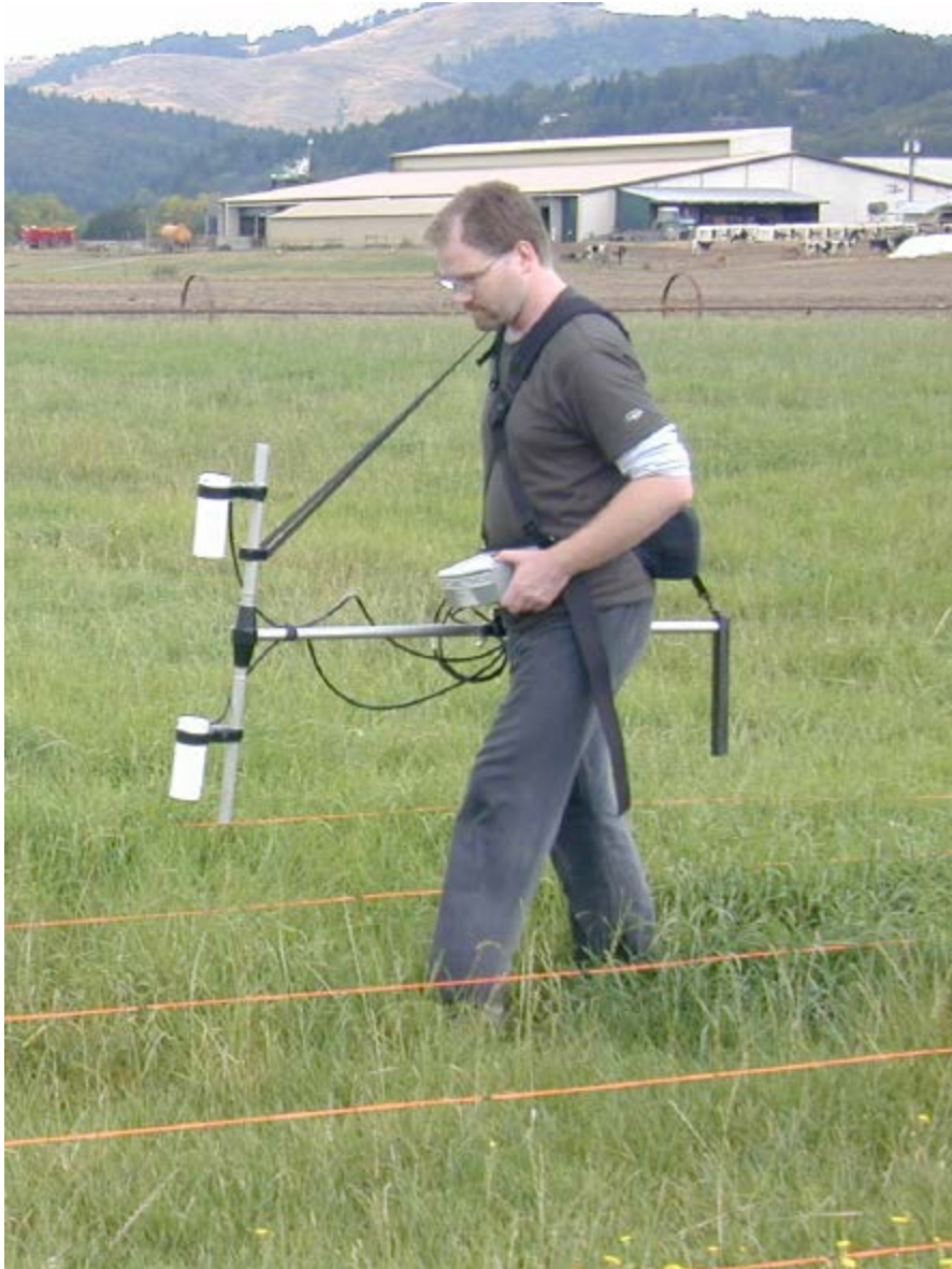
Figure 8. Cesium Vapor Total Field Magnetometer (CVTFM)
