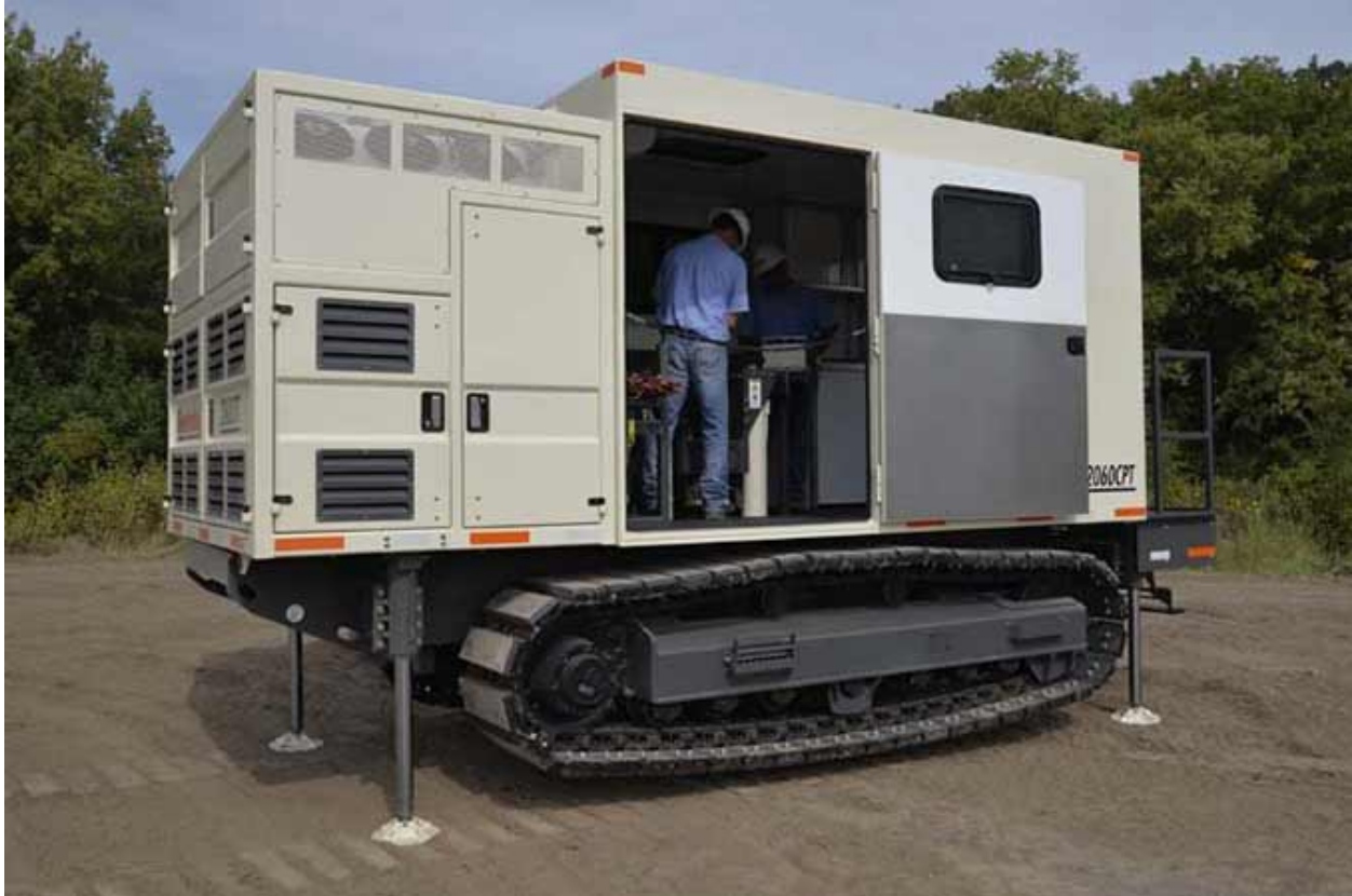
Figure 6. Track-Mounted Cone Penetrometer Testing Rig
