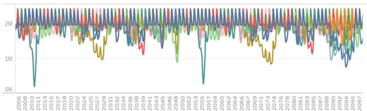
Figure 105 Future Projections of Monthly Storages in New Melones Reservoir, Single Urban Growth Scenario CTP-CTD, 20 Climate Scenarios, 2006–2100
