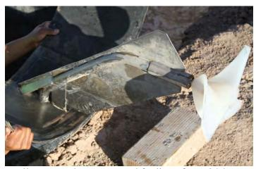
Figure 8. Propeller meter shows no weed fouling after a 24-hour run, using the propeller protection system, September 26-27, 2011.
